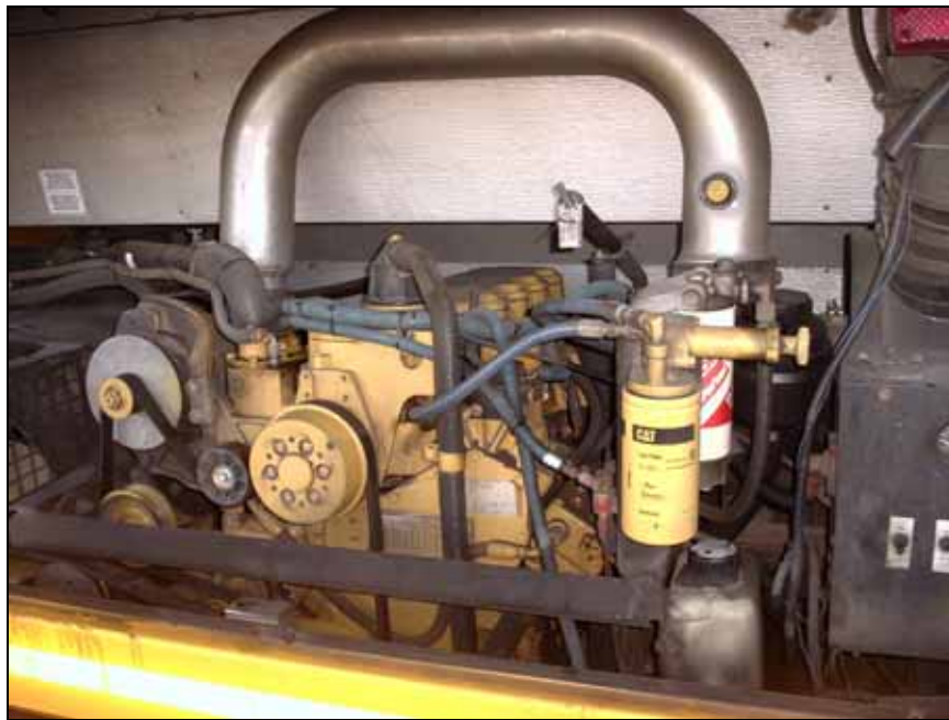
School Bus Engine – Arlington mechanics have experienced no mechanical problems that they can attribute to the adoption of B20
